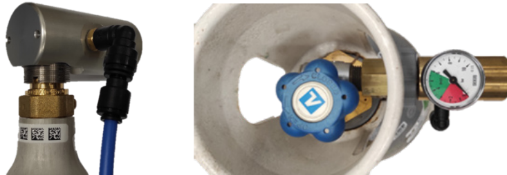
Figure 6.4.1 Connection of the pressure reducer - small pressure cylinder (left) and big pressure cylinder (right)
